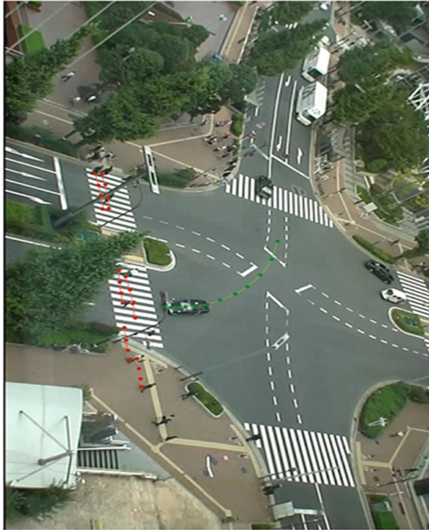
Fig. 9. Image captured from a camera installed at a high floor of a building around the intersection. The red points are the labeled pedestrian trajectories, and the green points are the labeled vehicle trajectories.
